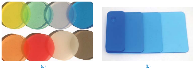
FIGURE 6: (a) Translucent palette of colored silicone. (b) The influence of thickness on color.
