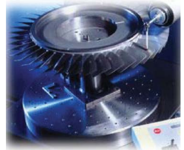
FIGURE 3: Titanium turbine blades during processing and fabrication.
