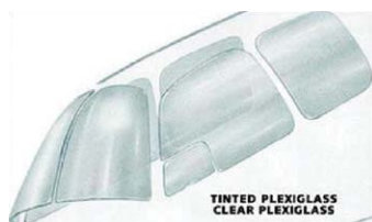
FIGURE 5: PMMA aircraft windshields are chosen for their excellent clarity and non-yellowing properties in outdoor environments. Silicones can be used to provide a seal around the windshield.
