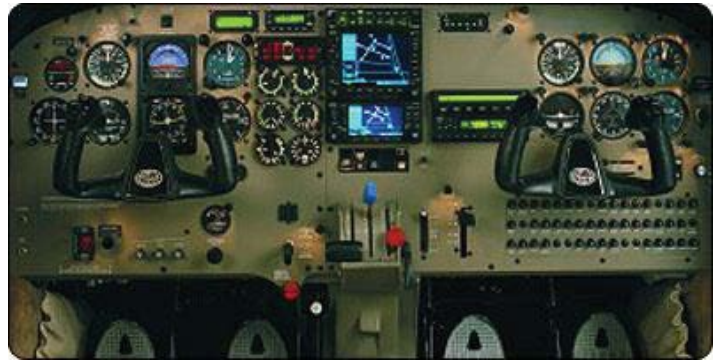
FIGURE 1: Aircraft cockpit showing Polyamide flight controls, PMMA displays, and polycarbonate & PEI flight consoles. Silicone adhesives can be used to seal the various components.
