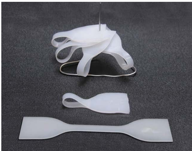
FIGURE 1: This image shows how tensile bars are shaped, folded and skewered onto the stainless steel wire.
