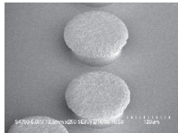
AFTER TREATMENT WITH J.T.BAKER BRAND PRS-3000 STRIPPER IN BATH AT 65°C, 20 MIN.
