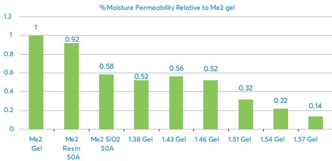
FIGURE 5: Phase 1 and 2 Analysis: Filler and chemical composition relative to Me2 gel
