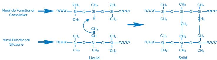
FIGURE 2. Crosslink Reaction
