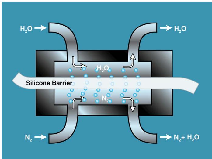
FIGURE 3. NuSil Interpretation of Mocon Isostatic Permeation Cell
