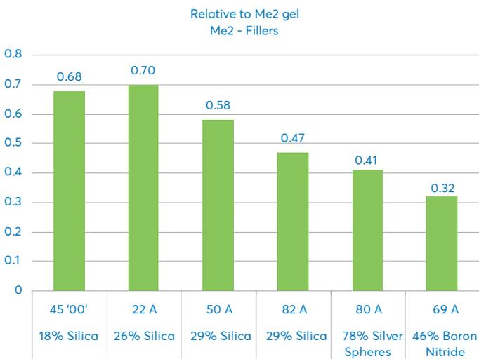
FIGURE 6: Relative Permeability Rates of filled systems Silica, Silver, Boron Nitride
