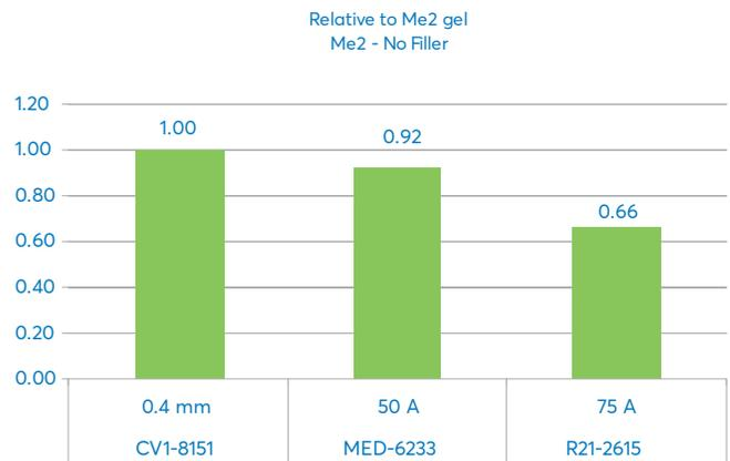
FIGURE 7: Relative Permeability Rates of PDMS to Me2 Gel: No Filler, Different Hardness
