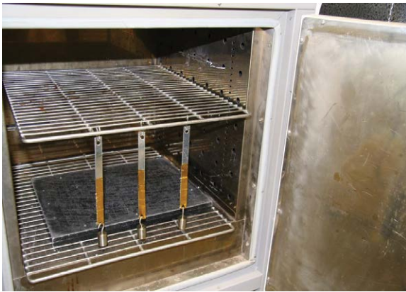
FIGURE 5: Static Shear Test; PSA coated onto Kapton and bonded to aluminum panels.
